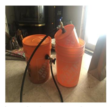
What: For our climate change action, we created an mini DIY anaerobic digester. Anaerobic digesters intake compost and food scraps to produce biogas, which mostly consists of methane gas. They do this by depriving bacteria of oxygen, therefore forcing them to digest the compost anaerobically and produce methane gas.
